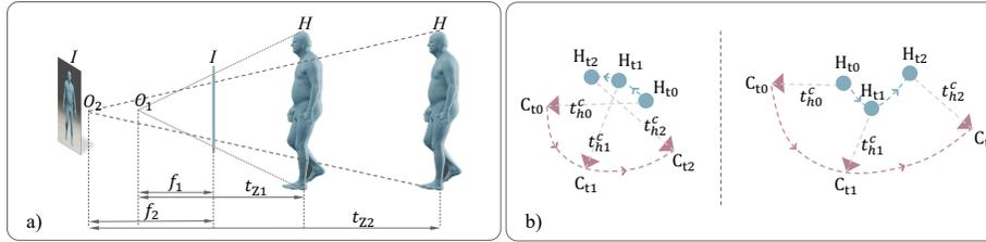
**Fig. 3:** a) Different pairs of focal length  $f$  and  $t_z$  can correspond to the same image. b) Human trajectories  $H$  derived from camera trajectories  $C$  of different scales can be vastly different in both shape and direction, despite that the same camera-frame human root translations  $t_h^c$  are used.
