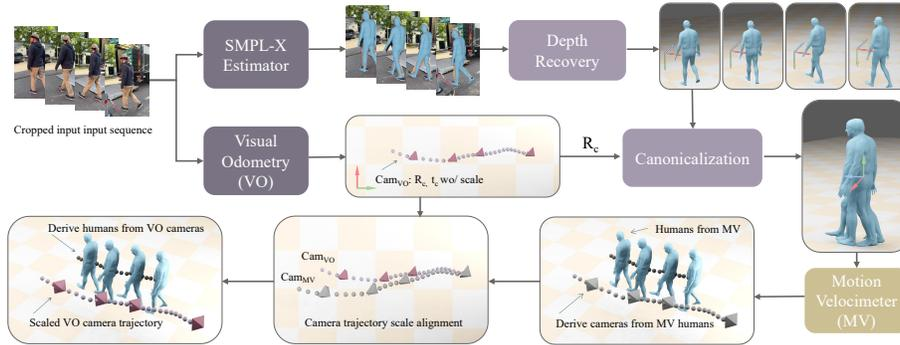
**Fig. 2:** Overview of **WHAC**. SMPL-X estimator extracts camera-frame SMPL-X with dummy depth [5], which is recovered in Sec. 3.2. The scaleless camera trajectory estimated by VO [39] is then used to canonicalize the human trajectory to estimate its velocity and thus scale in Sec. 3.3. A camera trajectory is then derived for alignment and scale recovery, which subsequently updates the human trajectory in Sec. 3.4.
